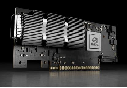
The NVIDIA® ConnectX®-7 family of remote direct-memory access (RDMA) network adapters supports InfiniBand and Ethernet protocols and a range of speeds up to 400 gigabits per second (Gb/s). It enables a wide range of advanced, scalable, and secure networking solutions that address traditional enterprise needs up to the world's most demanding AI, scientific computing, and hyperscale cloud data center workloads.
