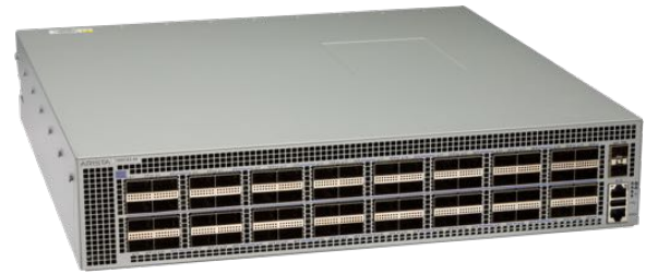
Arista 7260CX3-64: 64x 100GbE QSFP100 ports, 2 SFP+ ports
